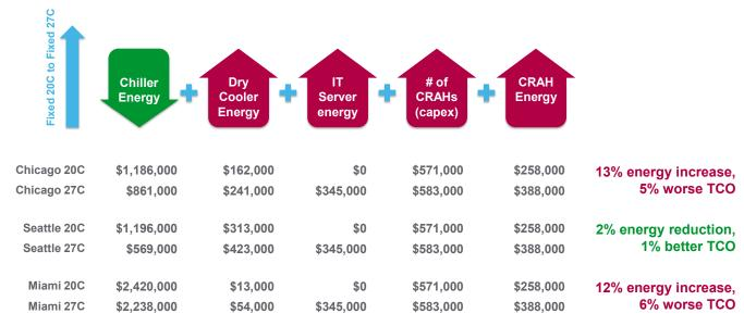
**Table 2** summarizes additional findings including total energy (kWh), and pPUE. Again, this illustrates that (1) energy is not always improved when you raise IT temperatures, and (2) PUE as a metric alone is insufficient.
