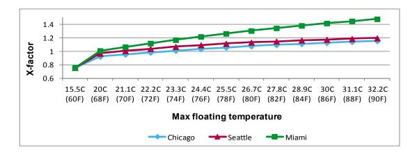
When comparing the baseline scenario to the higher fixed temperature of 27°C (80°F), there is a **31% increase in failures**. This is regardless of location, because now, the IT equipment is exposed to the same higher temperature year-round.
