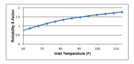
This data illustrates that, relative to the failure rate of servers at 20°C (68°F), there will be an increase in failures as the operating temperature rises. Therefore, simply raising a FIXED set point temperature will always decrease reliability if the servers follow the curve of **Figure 7**.
