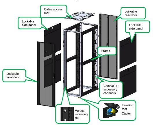
Figure 2 Three dimensional exploded view of a typical IT rack
