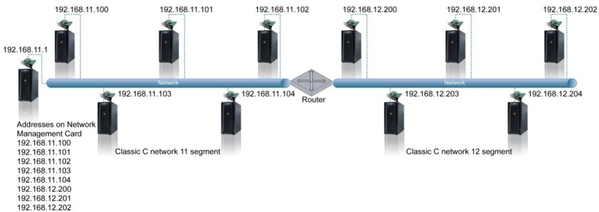
Figure 1 All 11 segment computers (192.168.11.xxx) will receive broadcasted UPS data while PowerChute computers on the 12 segment (192.168.12.xxx) will receive unicast UPS data every 25 seconds.
