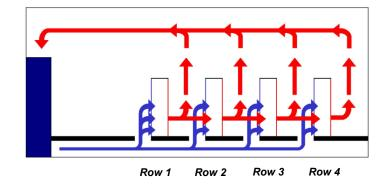
Best practice is to configure equipment in alternating "hot" and "cold" aisles as shown in Figure 8. Cold aisles contain the vented floor tiles, and racks are arranged so that all server fronts (intakes) face a cold aisle. Hot air exhausts into the hot aisle, which contains no vented floor tiles.
