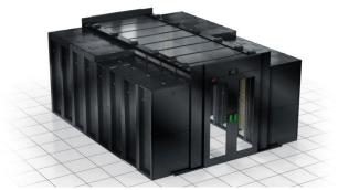
For high density zones, a hot aisle containment system (HACS) can be deployed to contain the hot aisle. Ceiling panels enclose the top of the row, while a set of end doors are used to contain the end of the hot aisle. Hot air from the servers (up to 60 kW per rack) is discharged into the contained hot aisle and drawn through the cooling unit to be discharged back into the room at ambient temperature.
