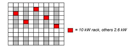
The fundamental reason why spreading out high-density loads is effective is because isolated high power racks can effectively "borrow" underutilized cooling capacity from neighboring racks. However, this effect cannot work if the neighboring racks are already using all the capacity available to them.
