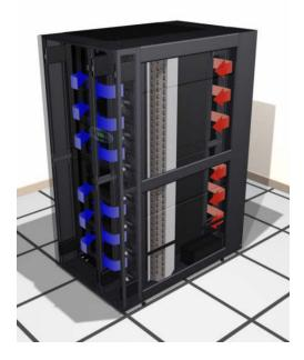
In a rack air containment system (RACS), single or multiple row-based cooling systems are tightly coupled with the IT enclosure, ensuring the maximum effectiveness of heat removal and cool air delivery to the rack-based equipment. (Up to 60 kW per Rack)
