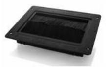
Missing floor tiles should be replaced and tiles reseated to remove any gaps. Cable cutouts in the floor cause the majority of unwanted air leakages and should be sealed around the cables using grommets (**Figure 4**). Tiles with unused cutouts should be replaced with full tiles. Tiles adjacent to empty or missing racks should also be replaced with full tiles.
