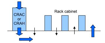
Note: Rack orientation may differ in some data centers. The example shown above is different from that illustrated earlier in **Figure 10**, but is included to demonstrate the airflow pattern described above.
