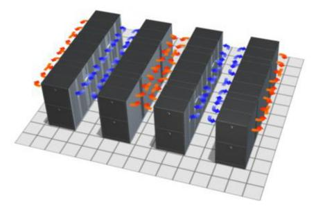
To further improve the efficiency and predictability of a row-based system, either rack or rowbased air containment systems can be added. These self-contained high-density cooling systems are designed to be installed in a data center without impacting any other racks or existing cooling systems. Such systems are thermally "room neutral" (or in many case, be thermally positive) and will take hot air from IT equipment, and discharge cool air back into the room, or enclosed cabinet.
