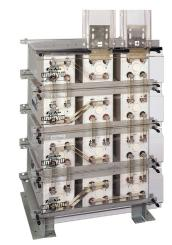
• "Battery cartridges" are actually multiples of VRLA batteries in a string conveniently packaged to allow their quick installation and removal. Battery cartridges can be plugged into battery cabinets designed with mating receptacles.
