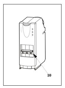
10 Set all breakers on the newly installed PDM to the ON (closed) position.
