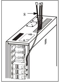
8 Feed cable from the PDM through the brush-filled slot in the roof of the PDU.
