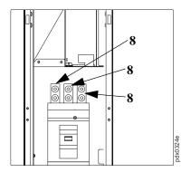
8 Connect the phase (L1, L2, L3) conductors. Torque: 31.1 Nm (275 lb-in).
