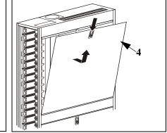
3 Open the safety door to expose the 4 input breaker.
