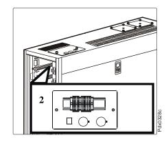
Note the location of the terminal block on the underside of a small top plate above the power distribution modules.
