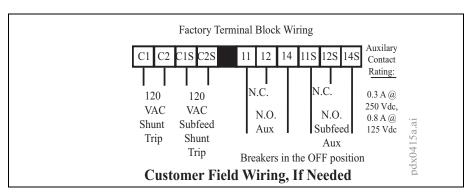
5 Make connections to appropriately labeled terminals on the terminal block.
