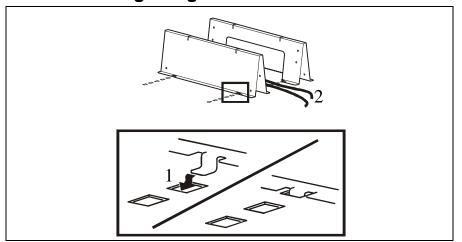
1 Snap an APC-provided trough into slots on the roof of the PDU. The tabs at the base of the trough must fit securely into the slots.
