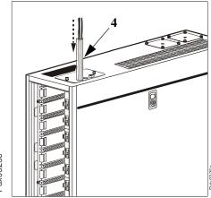
4 Attach conduit containing contact wires from external devices to the knockout.
