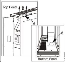
Loosen the screws from the mains shield and remove the shield to gain access to the compression terminals. Only remove the bottom shield if the bottom entry is used.
