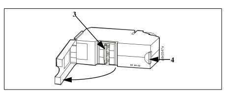
3 Make sure all breakers on the PDM that is being installed are in the **OFF** (open) position.
