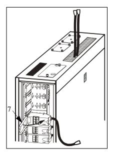
7 Close the latch. This will tighten electrical contacts in the PDM against the busbar.
