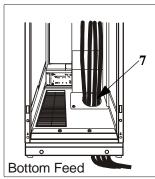
7 Install the conduit and pull the conductors into the PDU from the bottom or the top.
