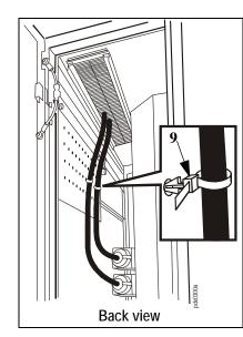
9 Use tie wraps to secure loose cables to the enclosure.
