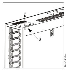
Working from inside the PDU enclosure, punch out the 64 mm (3/4 in) knockout in the small top plate.
