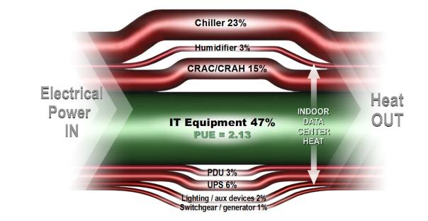
The energy consumption of a data center over a period of time is computed using the average of the data center efficiency over that period. Therefore, when we speak about data center infrastructure efficiency (PUE), we really are interested in the average efficiency over a period of time.
