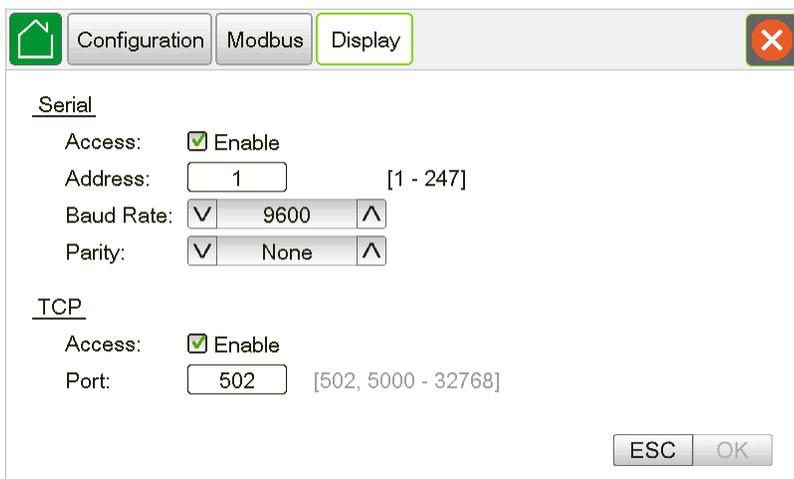
The screenshot shows a configuration window with three tabs: Configuration, Modbus, and Display. The Display tab is selected. Under the 'Serial' section, 'Access' is checked 'Enable', 'Address' is set to '1' (range [1 - 247]), 'Baud Rate' is set to '9600' (range [4800 - 19200]), and 'Parity' is set to 'None' (range [None - Even]). Under the 'TCP' section, 'Access' is checked 'Enable' and 'Port' is set to '502' (range [502, 5000 - 32768]). 'ESC' and 'OK' buttons are at the bottom right.
