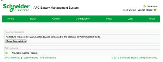
This page shows any *Active Alarms* for the system. This page also allows for the user to *Reset Annunciators*.
