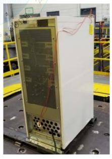
The UUT was rigid-base mounted using customer provided seismic kit (PN: GVSOPT002). The seismic kit mounting details can be found on the following page. M8 bolts were torqued to 21 Nm. M10 bolts were torqued to 42 Nm.
