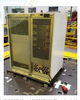
The UUT was rigid-base mounted using customer provided seismic kit (GVSOPT002 and GVSOPT008). The seismic kit mounting details can be found on the following page. M8 bolts were torqued to 21 Nm. M10 bolts were torqued to 42 Nm. Unit maintained structural integrity and remained functional per manufacturer requirement after shake table test. Contents were included in testing per operating conditions.
