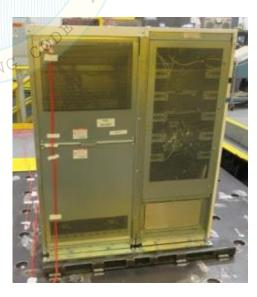
The UUT was rigid-base mounted using customer provided seismic kit (GVSOPT002 and GVSOPT008). The seismic kit mounting details can be found on the following page. M8 bolts were torqued to 21 Nm. M10 bolts were torqued to 42 Nm. Unit maintained structural integrity and remained functional per manufacturer requirement after shake table test. Contents were included in testing per operating conditions.
