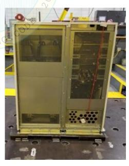
The UUT was rigid-base mounted using customer provided seismic kit (GVSOPT002 and GVSOPT008). The seismic kit mounting details can be found on the following page. M8 bolts were torqued to 21 Nm. M10 bolts were torqued to 42 Nm. Unit maintained structural integrity and remained functional per manufacturer requirement after shake table test. Contents were included in testing per operating conditions.
