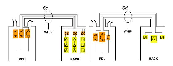
The analysis of this paper suggests that distribution whips that include single or 3phase 30 A whips are not preferred except in the case of dedicated whips. The 30 A whip value isn't optimal because the most common branch circuit size that must be generated in a rack is 20 A, which leads to two undesirable problems with a 30 A whip size:
