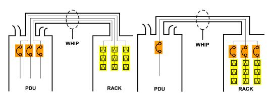
The arrangements of **Figure 5b** and **5c** are capable of providing the same power, but with a different wiring and circuit breaker arrangement. Note that in **Figure 5b**, the conduit or "whip"<sup>4</sup> contains multiple branch circuits. These alternatives give rise to significant advantages and disadvantages as summarized in **Table 2**.
