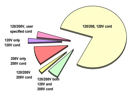
This complex situation suggests the need for the rack power distribution system to provide both 120 V and 208 V. However, it is possible to consider using a system restricted to a single voltage, either 120 V or 208 V. These two possibilities are discussed below.
