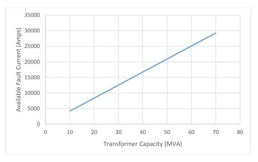
**Figure 9** Available fault current vs. transformer capacity, 13.8 kV distribution system
