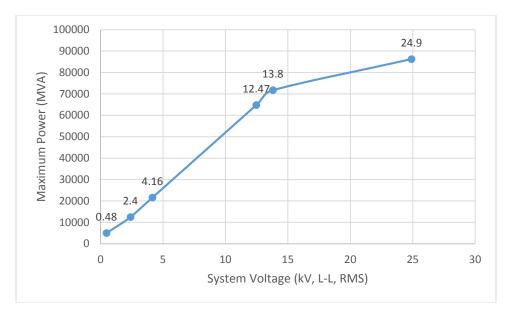
As shown, the capacity increases linearly through approximately 15 kV, and rises somewhat more slowly to 25 kV. While the additional capacity is desirable, there are some drawbacks associated with the move to higher distribution voltages, such as larger and more expensive equipment, at least when considered in absolute terms. If switchgear cost and footprint are considered on a per-kW basis, "economies of scale" at MV may become evident. The need for higher system capacity
