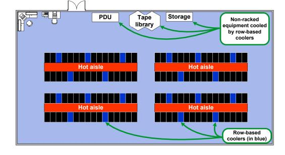
Sample data center layout with row cooling and ancillary IT equipment
