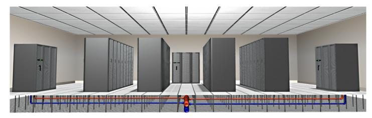
Traditional underfloor chilled water piping installation with branches to different air conditioners using multiple fittings
