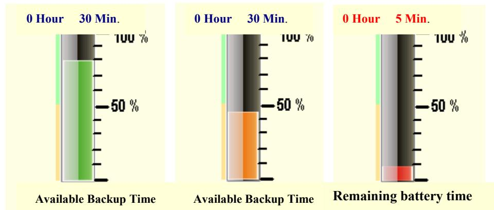
The "Available backup" and "Remaining backup" messages, located underneath the "bargraph", correspond to battery charging and discharging states respectively.
