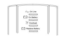
On Line (green) - is lit whenever utility power is powering the Battery Backup outlets.
