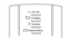
$\triangle$  On Line (green) - is lit whenever utility power is powering the Battery Backup outlets.
