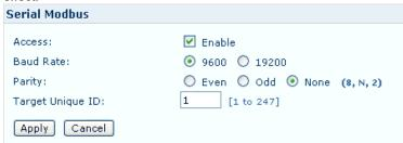
In case of AP9635 version 6.0 or higher or AP9641/43/44, navigate to Configuration >> Network >> Modbus
